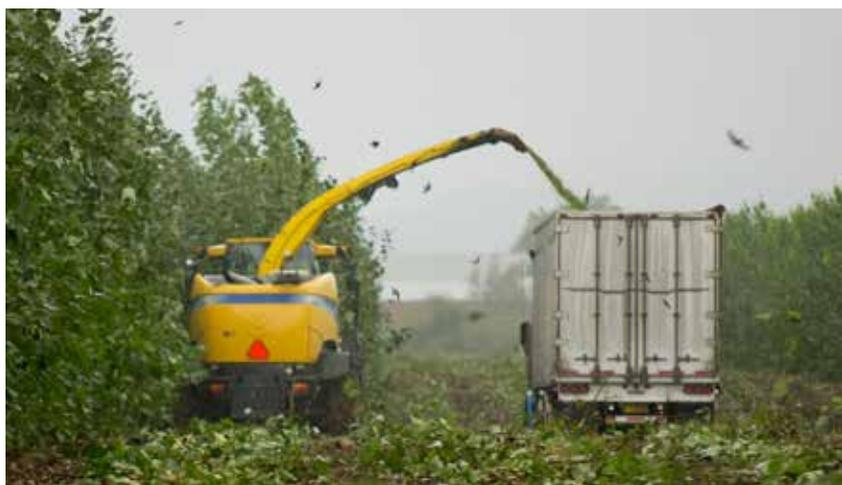
*A modified harvester cuts, chips, and blows hybrid poplar biomass into a truck that will haul it to a biofuel processor*
